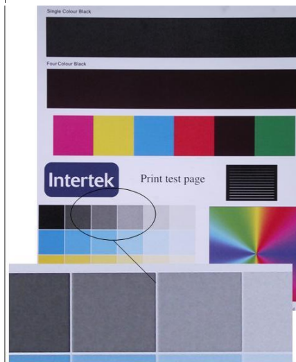
Close up of half tone black showing reduced mottle and higher density at optimum transfer current
