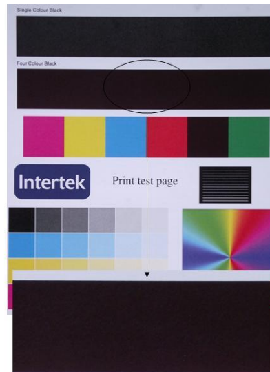
Close up of 4 colour black showing good print quality at the optimum transfer current
