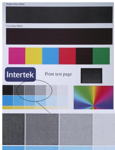
Close up of half tone black showing mottle caused by too low a transfer current
