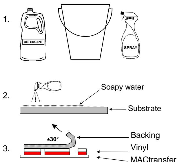
Prepare a solution of soapy water (one capful of detergent to 10 litres of water) and pour it into a spray bottle.
