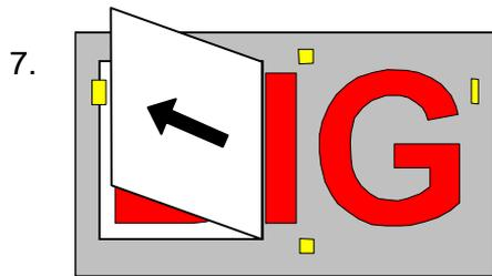
Remove the AT at a steady speed, at a cleaving angle of between 0 and 30°.
