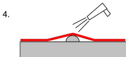
Heat MACfleet 6500 with a heat gun (at  $\pm 250$  °C). Squeeze out any air trapped between the MACfleet and the rivet using your finger.
