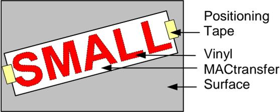
Place the application tape on top of the lettering or logo. Position the lettering or the logo **WITHOUT REMOVING THE BACKING**, using positioning tape at each end.
