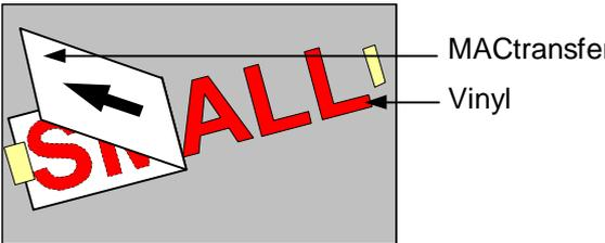
Pull the AT off at steady speed, at a cleaving angle of 0 to 30°. Prick any air bubbles (\*) trapped between the vinyl and the substrate.
