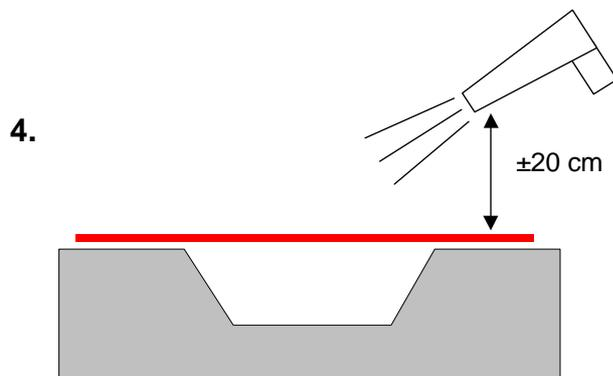
Heat MACfleet 6500 with an industrial air gun (air temperature: ±250°C).
