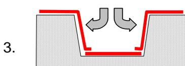
Apply the cut vinyl without tension in the corrugation.
