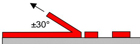
For best weeding results, use a cleaving angle of  $\pm 30^\circ$  and pull at a steady speed.
