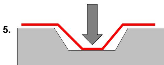
Press the vinyl into the corrugation using your finger covered by a cotton glove.
