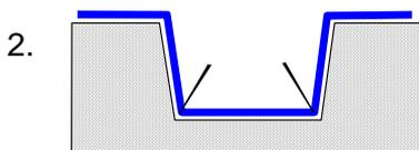
After the stabilisation process, let the film(s) cool down for 5 minutes and then cut the film(s) in the corrugation with a cutter in all the angles.
