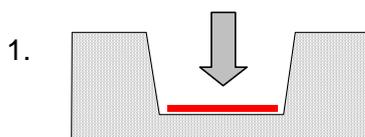
Before applying the decoration on the car, cut a strip of MACfleet 6500 (same colour as the one used in the decoration) and apply it without tension inside the corrugation.
