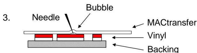
Turn the layers over and prick any air bubbles trapped between the application tape and the vinyl using a needle or a cutter (bubbles could cause wrinkling when applying the marking film on the substrate).
