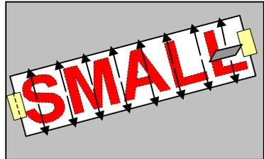
Position the lettering or the logo once again on the spot marked by the piece of positioning tape. Squeegee quickly and firmly from the centre outwards in overlapping movements.
