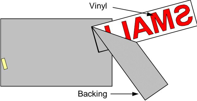
Cut one edge of the positioning tape. Peel the backing off.
