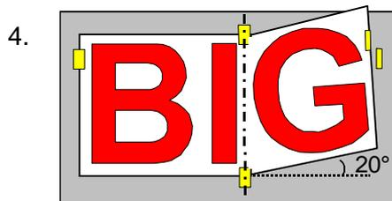
Fold the hinge back making sure that you leave a space between the MACfleet and the substrate surface (angle of  $\pm 20^\circ$ ) in order to avoid it sticking too soon.
