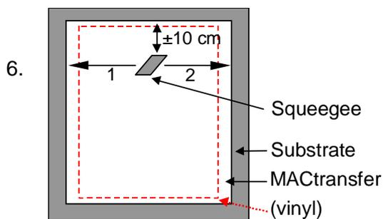
Squeegee horizontally, working from the centre outwards to the left and then the right stopping  $\pm 10$  cm from the top edge of the vinyl.
