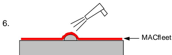
Finish off by stabilising the MACfleet with a heat gun (air temperature at  $\pm 650$  °C).
