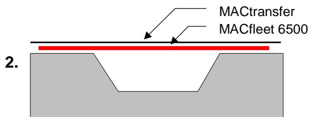
Apply MACfleet 6500 using MACtransfer application tape over the 3 dimensional surface.
