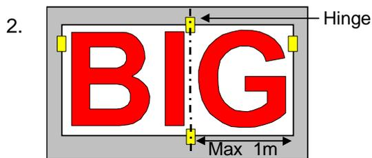
Make a hinge perpendicular to the largest dimension of the letters or logo, no more than 1m away from any one of the edges.
