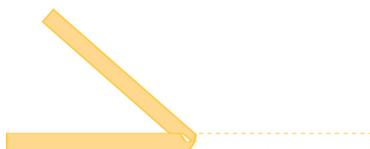
The molecules in the material become orientated as a result of this lengthening of the material. Priplak's® resistance is increased where the creases occur, and the hinge is as strong as the material made during manufacture.
