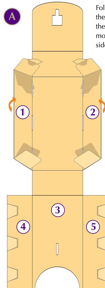
Fold both sides (1 and 2) inwards and take back the lower flap (3). Superimpose the sides (4 and 5) on the sides that are already folded, then slide the tabs into the slots. Two lateral grommets (6 et 7) provide a system of fixation without modifying the total look. Now, all that remains to be done is to fold the upper side (8) and close the box, sliding the clasp (9).
