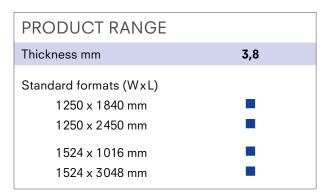
Tolerances: Thickness  $\pm 0.4$  mm. Width and length  $\pm 5$  mm. The given measurements are standard dimensions, ex works. Special sheet sizes upon request, cut to size sheets are available from your distributor.
