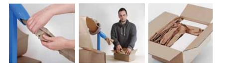
The simple design of the converter allows anyone to shape the single layer paper effectively into a filling material to protect products during shipment. No electricity is needed, and the labor-intensive hand crumpling of paper is eliminated. The fanfolded packs of paper offer easy handling, a minimal loading time and less storage costs. The paper is perforated every 18.6cm, allowing the operator to adjust the paper length to fit every void.
